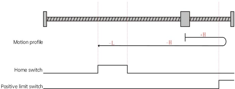
The current position of the motor is where the home switch is active. When the homing is started, the home switch is at high level, and the motor runs in the reverse direction at low speed, and stops when reaching the falling edge of the home switch.
