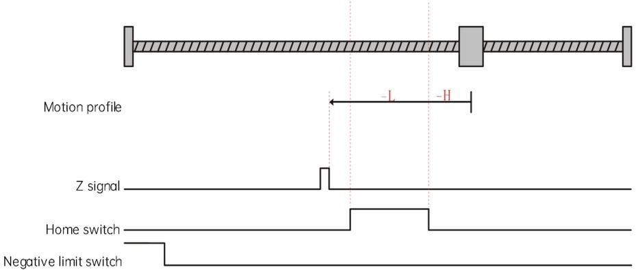
The current position of the motor is between the negative limit switch and the home switch. When the homing is started, the home switch is at low level, and the motor starts homing in the reverse direction at high speed. After reaching the rising edge of the negative limit switch, the motor runs in the forward direction at high speed. After reaching the rising edge of the home switch, the motor runs in the reverse direction at low speed, and stops when reaching the rising edge of the Z signal.
