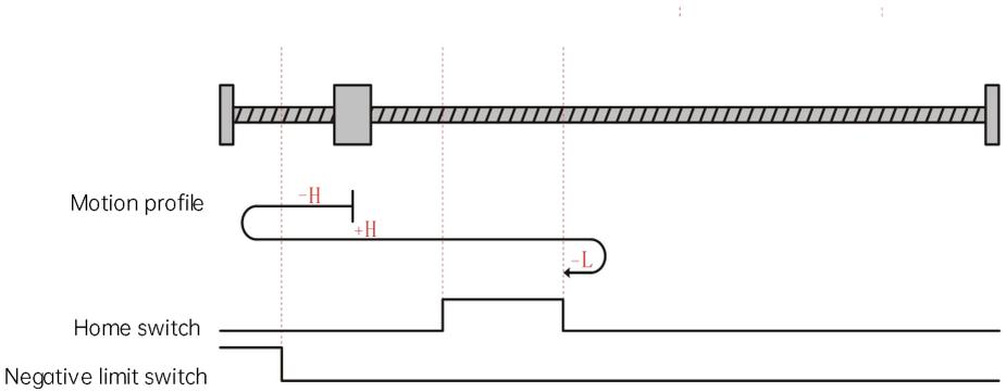
The current position of the motor is where the home switch is active. When the homing is started, the home switch is at high level, and the motor starts homing in the forward direction at high speed. After reaching the falling edge of the home switch, the motor runs in the reverse direction at low speed, and stops when reaching the rising edge of the home switch.
