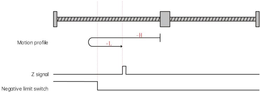
The current position of the motor is at the negative limit switch. When the homing is started, the negative limit switch is at high level, and the motor starts homing in the forward direction at low speed. After reaching the falling edge of the negative limit switch, the motor runs in the forward direction at low speed, and stops when reaching the rising edge of the Z signal.
