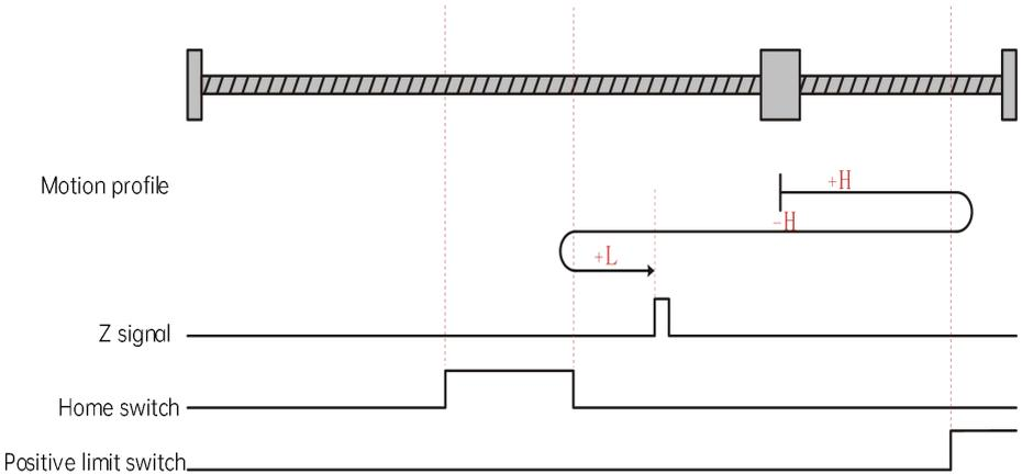
The current position of the motor is where the home switch is active. When the homing is started, the home switch is at high level, and the motor starts homing in the forward direction at low speed, and stops when reaching the rising edge of the Z signal.
