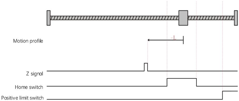
The current position of the motor is between the positive limit switch and the home switch. When the homing is started, the home switch is at low level, and the motor starts homing in the forward direction at high speed. After reaching the rising edge of the positive limit switch, the motor runs in the reverse direction at high speed. After reaching the rising edge of the home switch, the motor runs in the reverse direction at low speed, and stops when reaching the rising edge of the Z signal.
