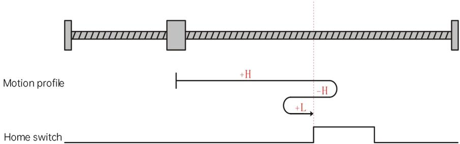
The current position of the motor is where the home switch is active. When the homing is started, the home switch is at high level, and the motor starts homing in the reverse direction at high speed. After reaching the falling edge of the home switch, the motor runs in the forward direction at low speed, and stops when reaching the rising edge of the home switch.
