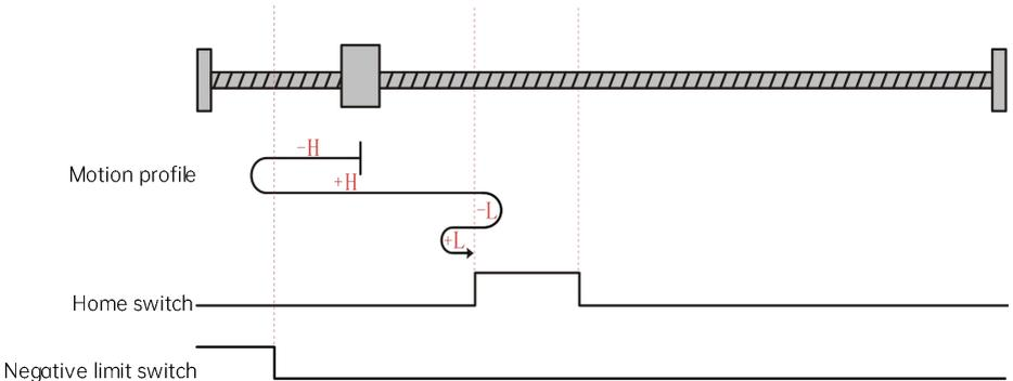
The current position of the motor is where the home switch is active. When the homing is started, the home switch is at high level, and the motor runs in the reverse direction at low speed. After reaching the falling edge of the home switch, the motor runs in the forward direction at low speed, and stops when reaching the rising edge of the home switch.
