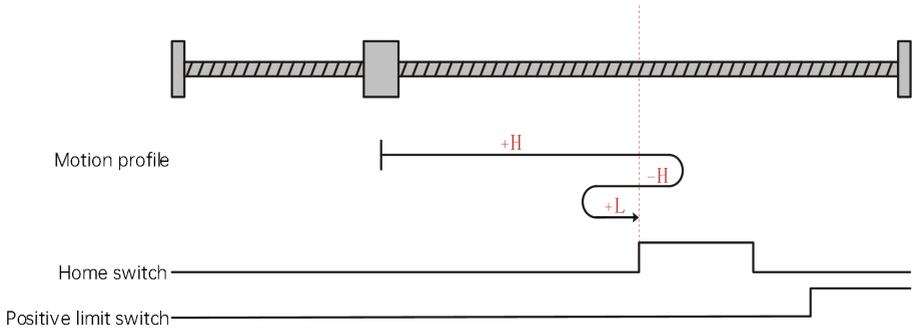
The current position of the motor is between the home switch and the positive limit switch. When the homing is started, the home switch is at low level, and the motor starts homing in the forward direction at high speed. After reaching the positive limit switch, the motor runs in the reverse direction at high speed. After reaching the falling edge of the home switch, the motor runs in the forward direction at low speed, and stops when reaching the rising edge of the home switch.
