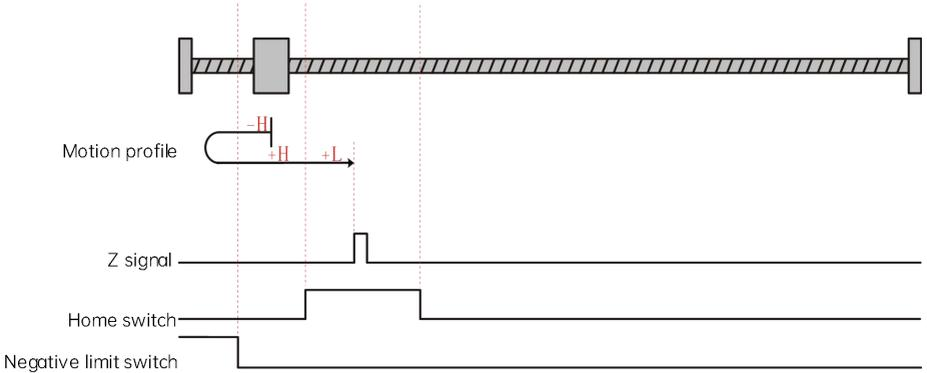
The current position of the motor is where the home switch is active. When the homing is started, the home switch is at high level, and the motor starts homing in the reverse direction at high speed. After reaching the falling edge of the home switch, the motor runs in the forward direction at high speed. After reaching the rising edge of the home switch, the motor runs in the forward direction at low speed, and stops when reaching the rising edge of the Z signal.
