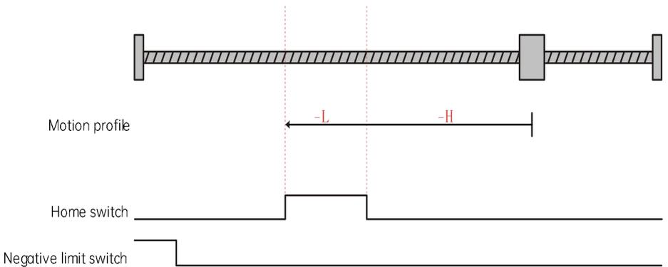
The current position of the motor is between the negative limit switch and the home switch. When the homing is started, the home switch is at low level, and the motor runs in the reverse direction at high speed. After reaching the rising edge of the negative limit switch, the motor runs in the forward direction at high speed. After reaching the rising edge of the home switch, the motor runs in the reverse direction at low speed, and stops when reaching the falling edge of the home switch.
