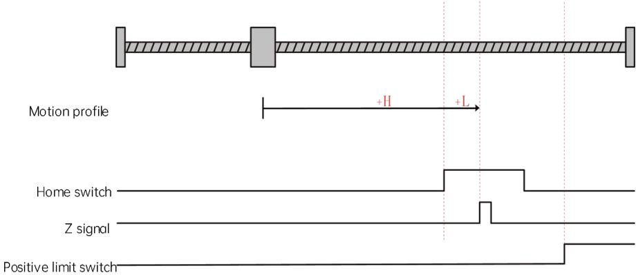
The current position of the motor is where the home switch is active. When the homing is started, the home switch is at high level, and the motor starts homing in the reverse direction at high speed. After reaching the falling edge of the home switch, the motor runs in the forward direction at high speed. After reaching the rising edge of the home switch, the motor runs in the forward direction at low speed, and stops when reaching the rising edge of the Z signal.
