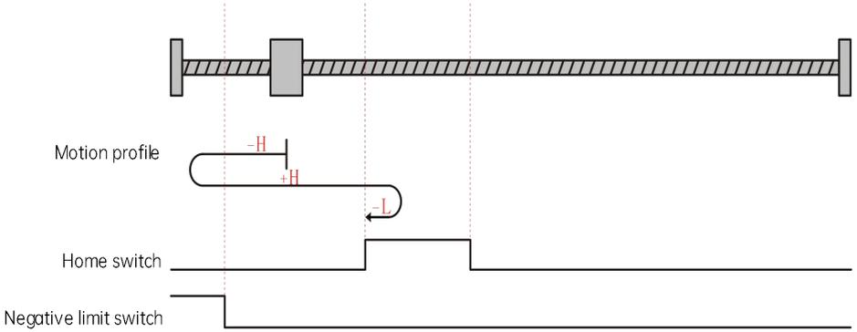
The current position of the motor is where the home switch is active. When the homing is started, the home switch is at high level, the motor runs in the reverse direction at low speed, and stops when reaching the falling edge of the home switch.
