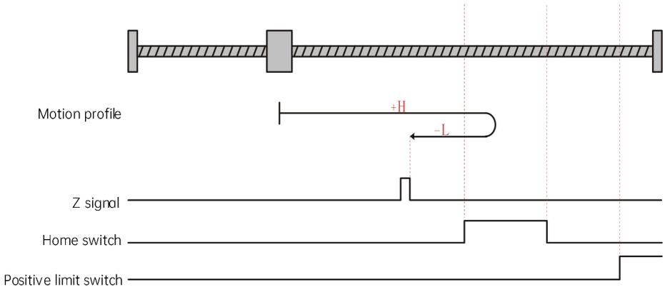
The current position of the motor is where the home switch is active. When the homing is started, the home switch is at high level, and the motor starts homing in the reverse direction at low speed. After reaching the falling edge of the home switch, the motor runs in the reverse direction at low speed, and stops when reaching the rising edge of the Z signal.
