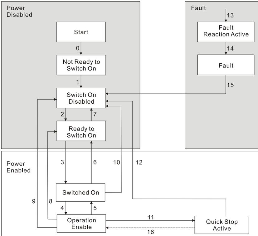
As shown in the diagram, the state machine consists of three main sections: "Power Disabled", "Power Enabled", and "Fault".
