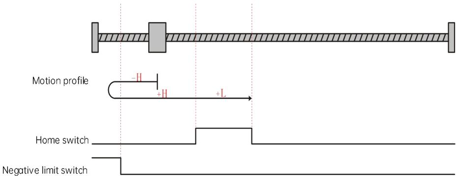
The current position of the motor is where the home switch is active. When the homing is started, the home switch is at high level, and the motor runs in the forward direction at low speed, and stops when reaching the falling edge of the home switch.
