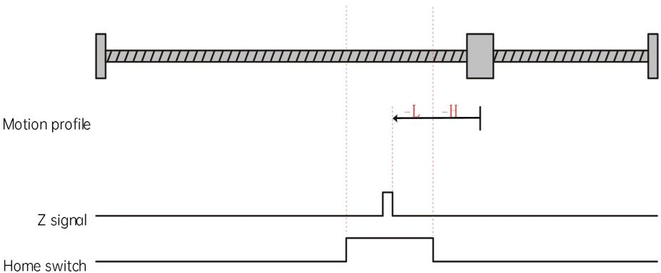
The current position of the motor is where the home switch is active. When the homing is started, the home switch is at high level, and the motor starts homing in the forward direction at high speed. After reaching the falling edge of the home switch, the motor runs in the reverse direction at high speed. After reaching the rising edge of the home switch, the motor runs in the reverse direction at low speed, and stops when reaching the rising edge of the Z signal.
