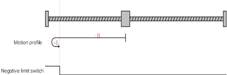
The current position of the motor is where the negative limit switch is active. When the homing is started, the negative limit switch is at high level, the motor runs in the forward direction at low speed, and stops when reaching the falling edge of the negative limit switch.
