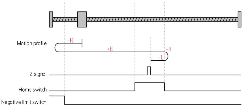
The current position of the motor is where the home switch is active. When the homing is started, the home switch is at high level, and the motor starts homing in the forward direction at high speed. After reaching the falling edge of the home switch, the motor runs in the reverse direction at high speed. After reaching the rising edge of the home switch, the motor runs in the reverse direction at low speed, and stops when reaching the rising edge of the Z signal.
