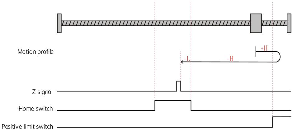
The current position of the motor is where the home switch is active. When the homing is started, the home switch is at high level, and the motor starts homing in the forward direction at high speed. After reaching the falling edge of the home switch, the motor runs in the reverse direction at high speed. After reaching the rising edge of the home switch, the motor runs in the reverse direction at low speed, and stops when reaching the rising edge of the Z signal.
