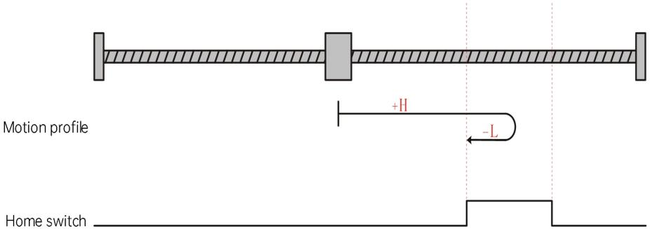
The current position of the motor is where the home switch is active. When the homing is started, the home switch is at high level, the motor runs in the reverse direction at low speed, and stops when reaching the falling edge of the home switch.
