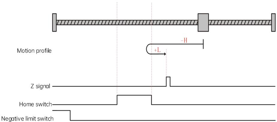
The current position of the motor is between the negative limit switch and the home switch. When the homing is started, the home switch is at low level, and the motor starts homing in the reverse direction at high speed. After reaching the rising edge of the negative limit switch, the motor runs in the forward direction at high speed. After reaching the rising edge of the home switch, the motor runs in the forward direction at low speed, and stops when reaching the rising edge of the Z signal.
