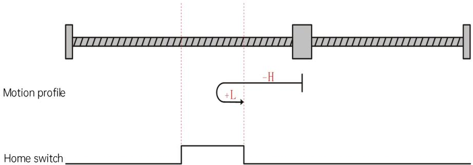
The current position of the motor is where the home switch is active. When the homing is started, the home switch is at high level, the motor runs in the forward direction at low speed, and stops when reaching the falling edge of the home switch.
