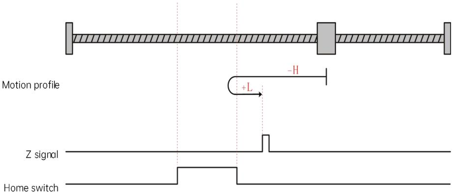
The current position of the motor is where the home switch is active. When the homing is started, the home switch is at high level, and the motor starts homing in the forward direction at low speed. After reaching the falling edge of the home switch, the motor runs in the forward direction at low-speed, and stops when reaching the rising edge of the Z signal.
