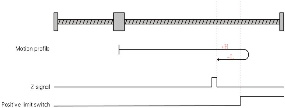
The current position of the motor is at the positive limit switch. When the homing is started, the positive limit switch is at high level, and the motor starts homing in the reverse direction at low speed. After reaching the falling edge of the positive limit switch, the motor runs in the reverse direction at low speed, and stops when reaching the rising edge of the Z signal.
