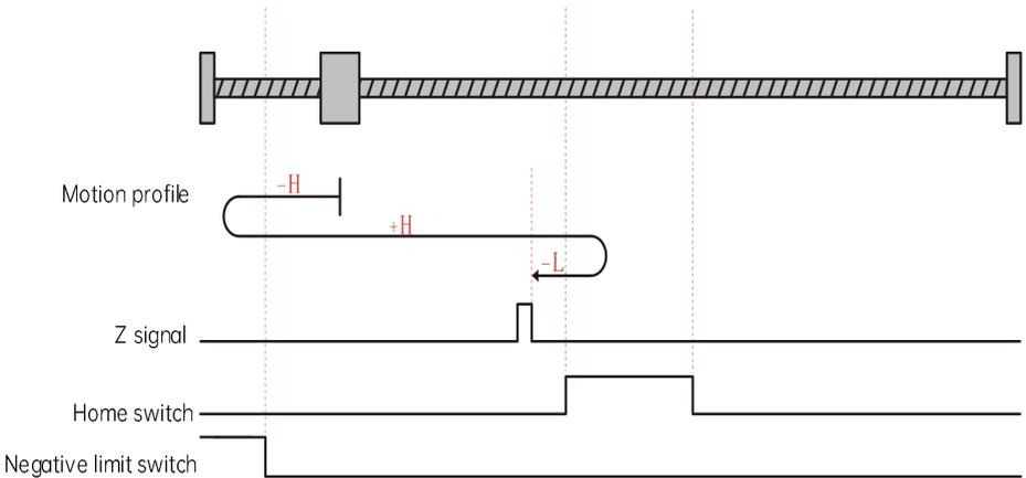
The current position of the motor is where the home switch is active. When the homing is started, the home switch is at high level, and the motor runs in the reverse direction at low speed, and stops when reaching the rising edge of the Z signal.
