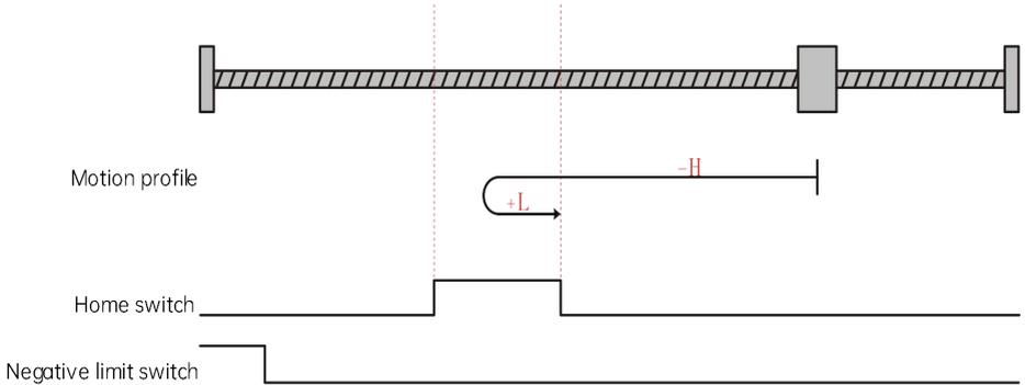
The current position of the motor is between the negative limit switch and the home switch. When the homing is started, the home switch is at low level, and the motor runs in the reverse direction at high speed. After reaching the rising edge of the negative limit switch, the motor runs in the forward direction at high speed. After reaching the rising edge of the home switch, the motor runs in the forward direction at low speed, and stops when reaching the falling edge of the home switch.
