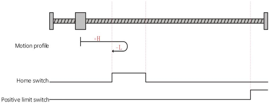
The current position of the motor is between the positive limit switch and the home switch. When the homing is started, the home switch is at low level, and the motor runs in the forward direction at high speed. After reaching the rising edge of the positive limit switch, the motor runs in the reverse direction at high speed. After reaching the rising edge of the home switch, the motor runs in the reverse direction at low speed, and stops when reaching the falling edge of the home switch.
