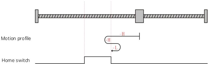
The current position of the motor is where the home switch is active. When the homing is started, the home switch is at high level, and the motor starts homing in the forward direction at high speed. After reaching the falling edge of the home switch, the motor runs in the reverse direction at low speed, and stops when reaching the rising edge of the home switch.
