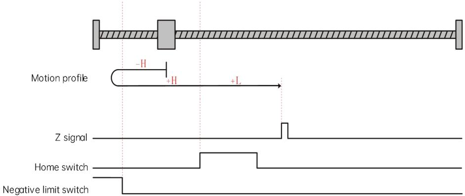
The current position of the motor is where the home switch is active. When the homing is started, the home switch is at high level, and the motor runs in the forward direction at low speed, and stops when reaching the rising edge of the Z signal.
