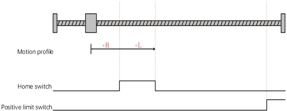
The current position of the motor is between the positive limit switch and the home switch. When the homing is started, the home switch is at low level, and the motor runs in the forward direction at high speed. After reaching the rising edge of the positive limit switch, the motor runs in the reverse direction at high speed. After reaching the rising edge of the home switch, the motor runs in the forward direction at low speed, and stops when reaching the falling edge of the home switch.
