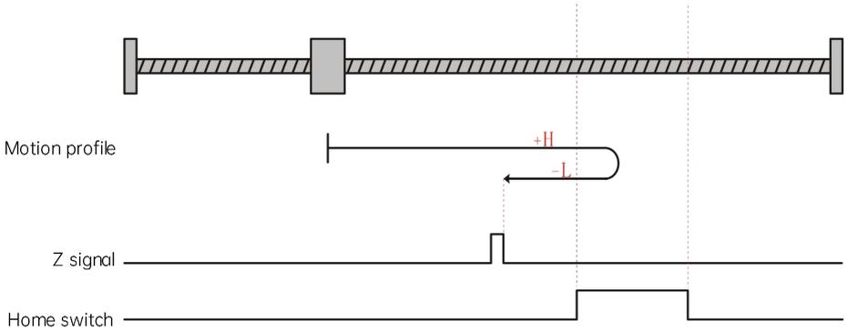
The current position of the motor is where the home switch is active. When the homing is started, the home switch is at high level, and the motor starts homing in the reverse direction at low speed. After reaching the falling edge of the home switch, the motor runs in the reverse direction at low speed, and stops when reaching the rising edge of the Z signal.
