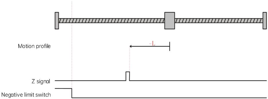
When the current position of the motor is at the Z signal, the homing enable is triggered, and the current position is immediately remembered as the home position to stop.
