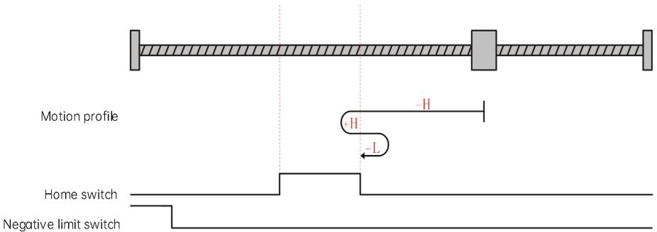
The current position of the motor is between the negative limit switch and the home switch. When the homing is started, the home switch is at low level, and the motor runs in the reverse direction at high speed. After reaching the negative limit switch, the motor runs in the forward direction at high speed. After reaching the falling edge of the home switch, the motor runs in the reverse direction at low speed, and stops when reaching the rising edge of the home switch.
