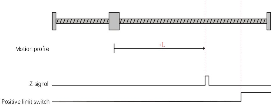
When the current position of the motor is at the Z signal, the homing enable is triggered, and the current position is immediately remembered as the home position to stop.
