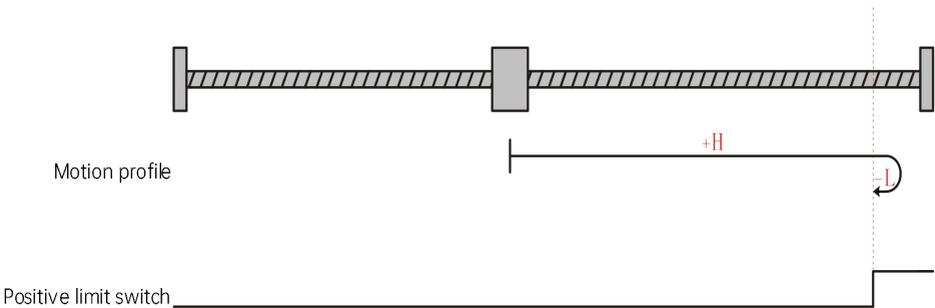
The current position of the motor is where the positive limit switch is active. When the homing is started, the positive limit switch is at high level, the motor runs in the reverse direction at low speed, and stops when reaching the falling edge of the positive limit switch.
