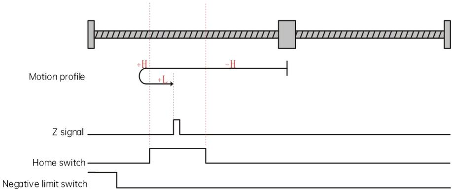
The current position of the motor is between the negative limit switch and the home switch. When the homing is started, the home switch is at low level, and the motor starts homing in the reverse direction at high speed. After reaching the rising edge of the negative limit switch, the motor runs in the forward direction at high speed. After reaching the rising edge of the home switch, the motor runs in the forward direction at low speed, and stops when reaching the rising edge of the Z signal.
