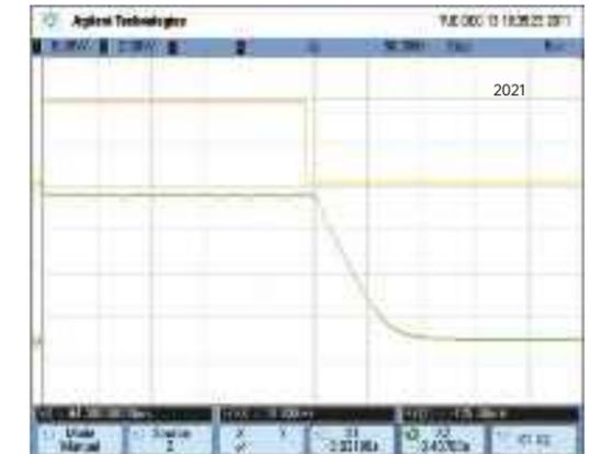
Unloading pressure time of 175 bar is less than 100 ms.
