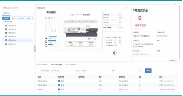
设备监控系统:设备状态监控、工艺参数获取、报警记录、历史数据、设备信息等。 Equipment monitoring system: equipment status monitoring, process parameter acquisition, alarm record, historical data, equipment information, etc.
